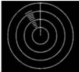
SART response from liferaft at medium range (2-3 miles). Note widening of "echos"
