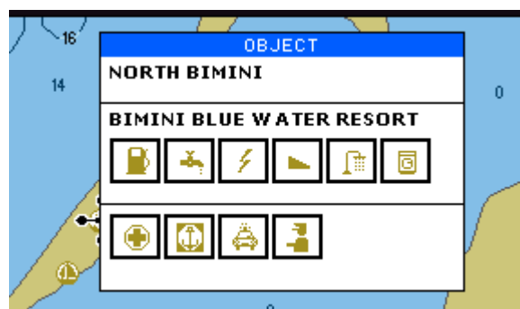
Sample filling station, service marks
